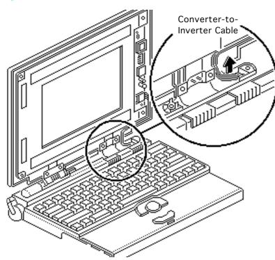
4 Remove the converterto-inverter cable from the case.
