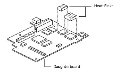
Using the Apple logic board take-apart tool, disconnect the daughterboard from the motherboard.
