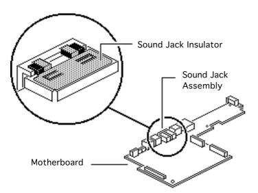
Replacement Note: To replace the insulator on the sound jack assembly, carefully peel off the original insulator. Remove the paper backing on the replacement insulator, and gently press it into place.
