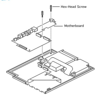
3 Remove the two hexhead screws and lift the motherboard from the bottom case.
