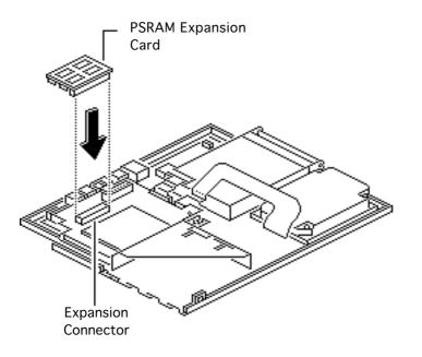
Connect the PSRAM expansion card to the expansion connector on the daughterboard.
