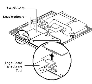
**Caution:** Always use the logic board take-apart tool to separate the cousin card connector from the daughterboard connector. Trying to disconnect the cousin card from the daughterboard by rocking or peeling the boards apart damages the connectors.
