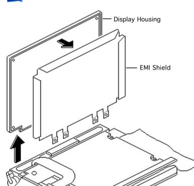
**Replacement Note:** Replace the short mounting screws in the top-inside clutch threadings. The top-outside threadings are used to mount the bezel.
