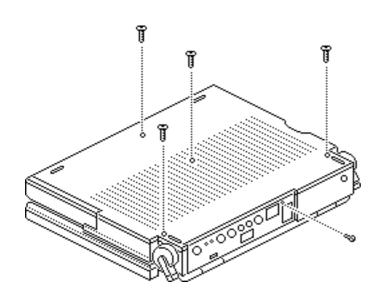
Note: Use a T-8 Torx driver to remove the small screw from the rear connector panel and a T-10 Torx driver to remove the other case screws.
