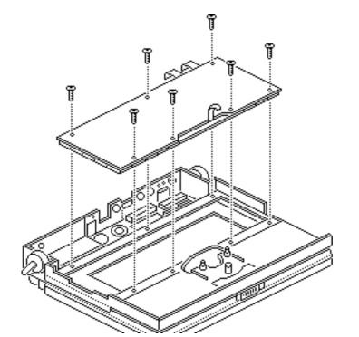
2 Using a T-8 Torx driver, remove the seven mounting screws and lift the keyboard from the top case.
