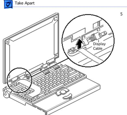
5 Remove the display cable from the case.
